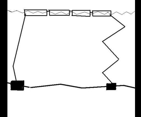
Under flood conditions, this is what happens. If the shorter anchor rope is on the downstream side, the last panel or 2 will be pulled under and turn upside down. Solution: always keep the shortest anchor rope on the upstream side.
