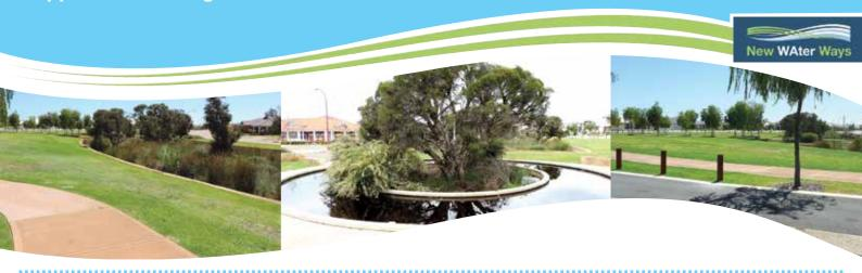
**Flowerfield Loop** borders a public open space (POS) area of Bletchley Park Estate which is characterised by a bioretention basin and retained native vegetation. The bioretention basin has been designed to treat local runoff generated during small rainfall events via native vegetation. The basin provides flood protection during rainfall events through detention of minor flows.
