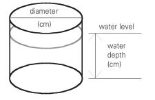
**FORMULA 1:** Volume (in litres) =  $0.8 \times \text{water depth (cm)} \times \text{diameter}^2 (\text{cm}^2) \div 1000$  (above diagram)
