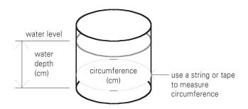
**FORMULA 2:** Volume (in litres) =  $0.08 \times \text{water depth (cm)} \times \text{circumference}^2 (\text{cm}^2) \div 1000$  (above diagram)
